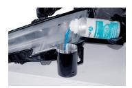
4. Add Headlight renovator polymer up to half of the vaporizer and cover with the lid that best suits the headlight shape.
